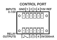
The control port on the rear of N8000 is divided into two parts. Two Phoenix connectors (6-pin) are included in delivery in order to be able to connect external components.
