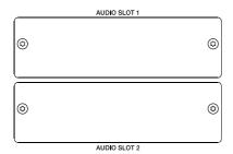
The AUDIO SLOTs 1 - 4 are module slots for the installation of NetMax audio modules. There are both analog and digital input and output modules available. Also, a module for microphone input sensitivity is optionally available. Each slot can accept any module so you can equip those inputs and outputs which you need for your specific application. The N8000 detects the type of the module automatically and offers the corresponding configuration possibilities.
