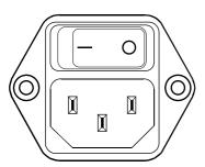
Please use the enclosed power cable in order to connect NetMax N8000 to the mains power supply. The N8000 is compatible with a supply voltage between 100 V AC and 240 V AC. Therefore, a supply voltage switch is not necessary. Internally, there is a mains fuse which is normally only blown in case of a fault. The fuse should only be replaced with an equivalent fuse with identical values for current, voltage and actuating characteristics by an authorized service center.
