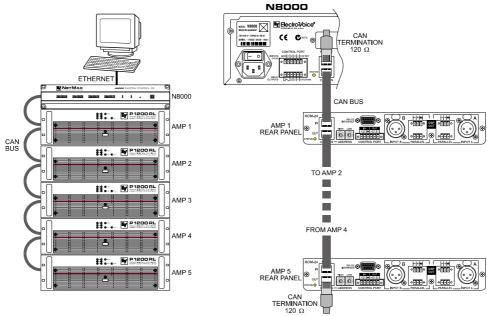
System with 5 power amps and 1 N8000 at the beginning of the bus. Termination plugs at the N8000 (first unit on the bus) and at amp 5 (last unit on the bus).
