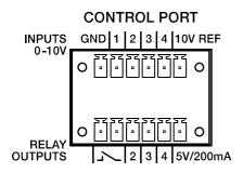
The CONTROL PORT contains four freely programmable control inputs, three freely programmable control outputs, one ready/fault output as well as reference connections for ground, +5 V and +10 V.
