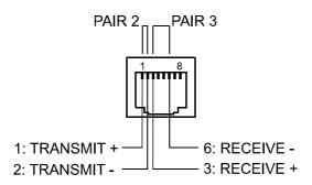
Pin Assignment of Ethernet jack
